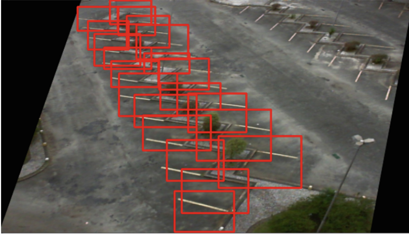
Fig. 9. Parking spaces plotted with unfiltered noise data
