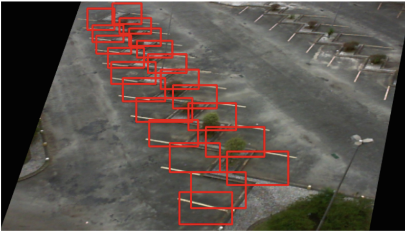
Fig. 10. Parking spaces plotted with filtered noise data
